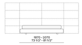
Two panels I 955 for mattress width I 1600 Two panels I 1037 for mattress width I 1800
