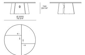
The arrows indicate the orientation of the wood grain.
